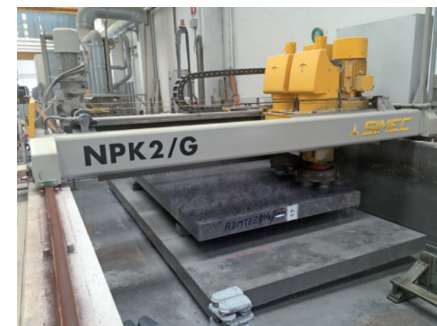
Lucidatrice a due mandrini modello NPK2/G. Two-spindle polishing machine model NPK2/G.
